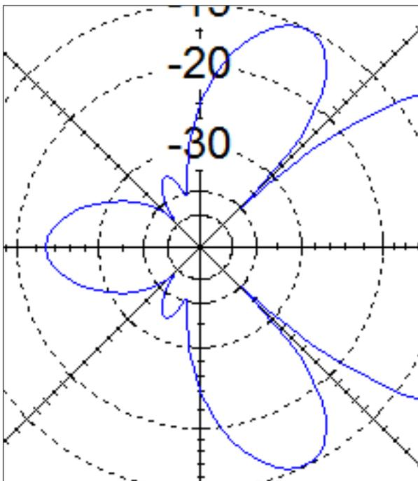
**Fig. 2c: The now balanced and symmetrical pattern of stacked LFA-Q Yagis result from switching the feed point position of each antenna to be a mirror-image of one another.**
